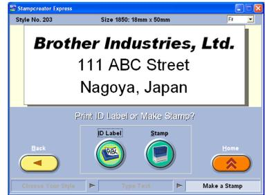
When the Print ID Label dialog box appears, check the stamp size, insert the appropriate ID label into the ID label slot of SC-2000USB, and then click the OK button.
